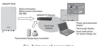
Fig. 7: Image of connection to "SANUPS PV Monitor"
