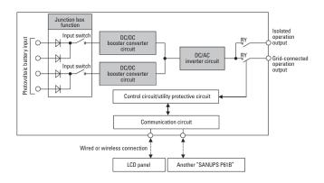
Fig. 4: Circuit block diagram (5 kW model)
