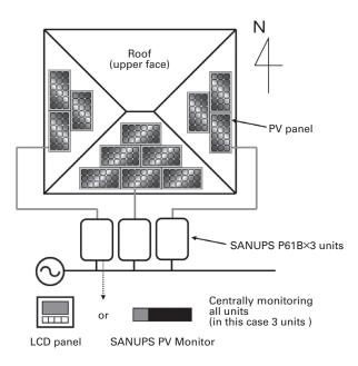
Fig. 5: Example of use as a string inverter
